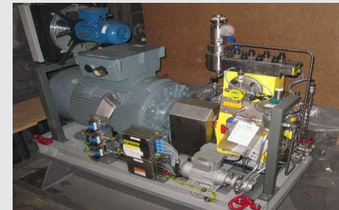
High pressure pumps
